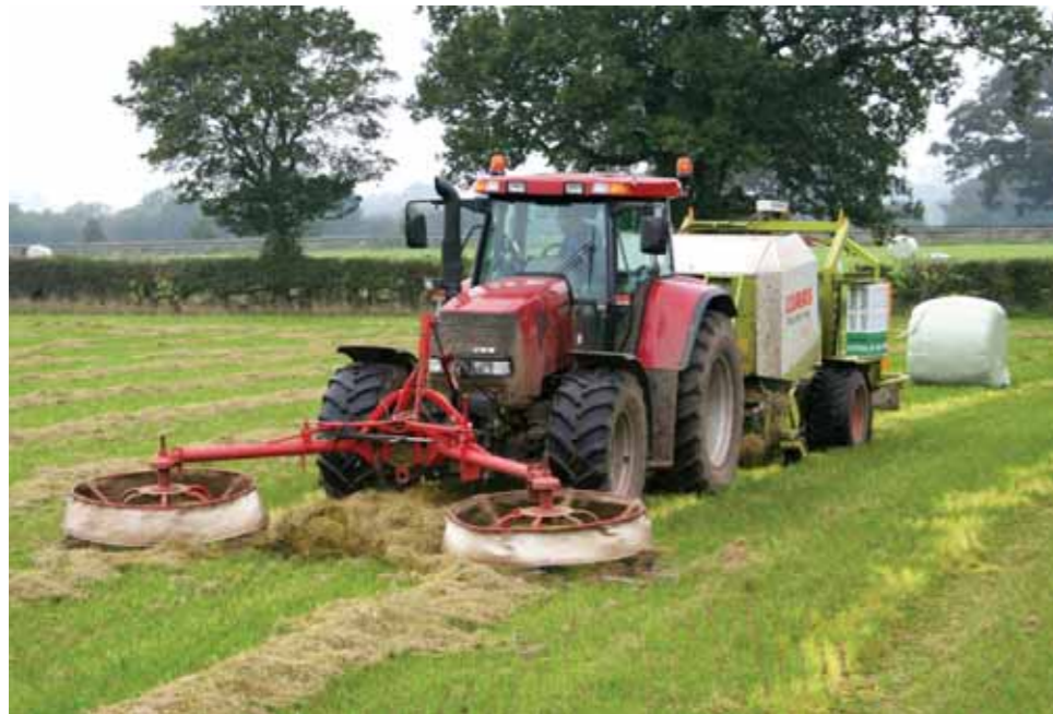
Above: Contractor Tim Walker raking a thin second-cut grass crop into a swath for baling and then wrapping – all in one pass. What a saving on time and fuel.
