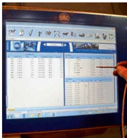
Control screen for the four robots is constantly monitored by staff to check how individual animals are performing and whether they're coming forward often enough for milking.
