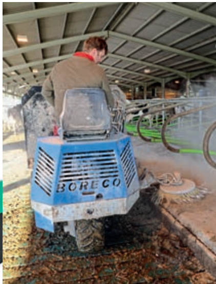
Keeping the heelstones clear with a rotating brush at the same time as applying limed paper bedding, the Boreco trike means it only takes 15 minutes to deal with all 400 cubicles.
