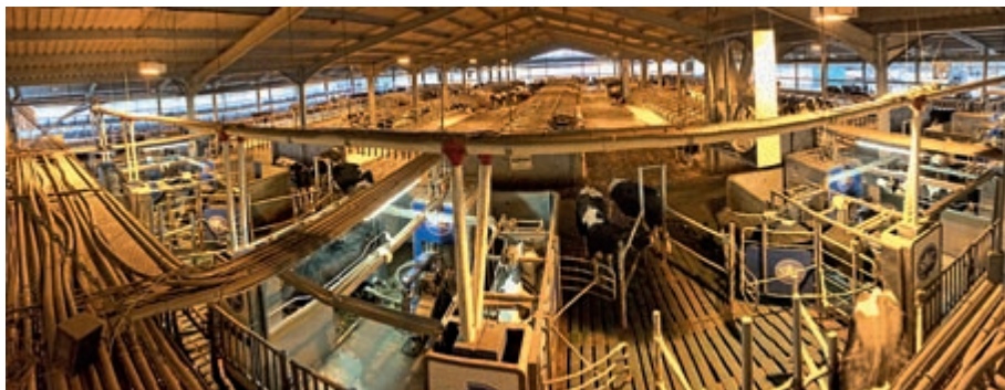
The four robots are arranged in a line across one wall of the three-span shed. To either side are holding pens for cows split out at the shedding gates with separate cubicles, water and feed.
