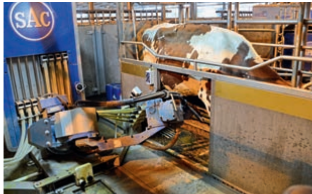
Generic Motorman robot arms of the sort used in car factories are employed in the SAC set-up. Their robust build was one of the main factors in choosing them, explains Max Frampton.
