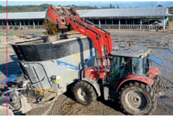
One of a brace of Massey 5480s fitted with loaders fills the mixer wagon. A JCB TM320-S pivot-steer has since taken over this role.
