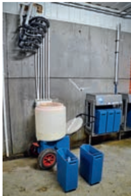
Mastitis milk is diverted automatically by the robots to a dump bucket.
