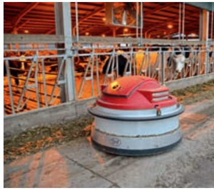
A Lely Juno feed pusher robot replaced a troublesome Joz Mooov for nuzzling fresh feed up to the barrier every two hours.
