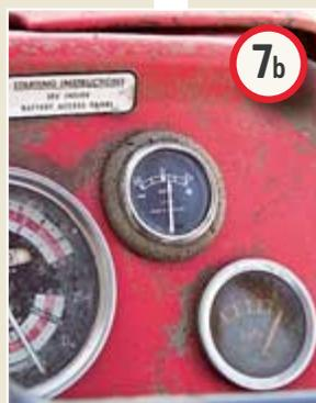
The dynamo or alternator drive belt needs to be in good order and tensioned properly; around 19mm (3/4in) deflection mid-way down a long belt run is good (7a). Slacken the unit's top pivot bolts a little, loosen the single anchor bolt underneath and swing it to adjust. Use a voltmeter or the tractor's ammeter to confirm a healthy charge (7b); a voltmeter connected between the battery terminals should show 13.5V-14.2V at medium rpm.
