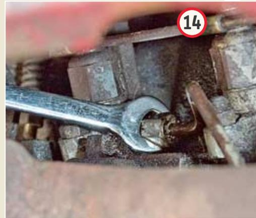
Follow each injector pipe up past the exhaust manifold; you're looking for the union nut where it joins the injector at cylinder head level. Using a short spanner, slacken each nut by a couple of flats.
