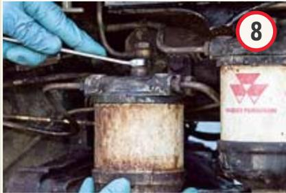
Before changing fuel filters, turn off the tank tap. If the tractor has a sedimenter – a primary dirt/water trap, usually with glass-bottomed bowl – clean it now. Tighten the glass bowl firmly as you don't want any air to be drawn in later. Then undo the filter(s).
