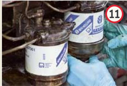
Fit the new filters, using the smaller square-section ring seal between filter and base. Tighten the holding bolt firmly, but don't go bananas or you'll do damage.
