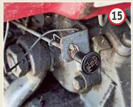
With the stop control in the 'run' position and the hand throttle opened up wide, spin the engine on the starter in ten second bursts until you see bubble-free fuel pulsing from the injector unions. **Caution:** Look but never touch – high-pressure fuel injected into the skin has extremely unpleasant consequences. Tighten the unions and try starting the engine. If it doesn't fire up, bleed again.
