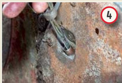
Transmission dipstick lives on the offside of the tractor, just ahead of the back axle. Oil should be up to the mark. If not, top up with a big-name brand Universal.
