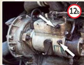
Start the air-bleed procedure by finding the lift pump (a) and injector pump bleed screws (arrows, b). On a 135 the lift pump is on the offside, the injector pump on the near.
