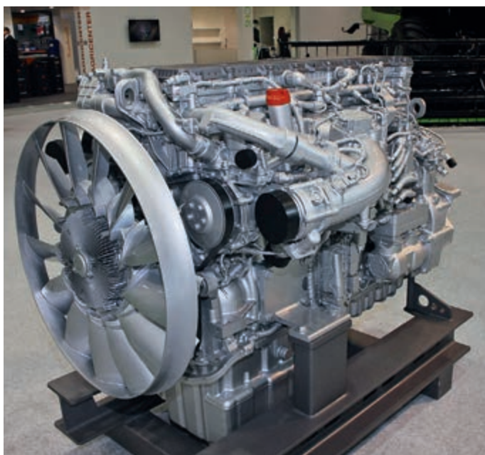
One of the latest engines to be developed by Deutz is this 12.8-litre, six-cylinder motor, which is turbocharged, intercooled and uses EGR with SCR exhaust after-treatment to achieve Stage IV emission control. Electronic engine management not only results in more efficient power delivery but also reduced fuel consumption, says Deutz.
