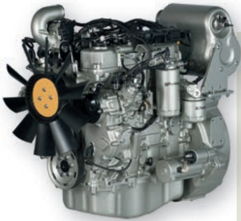
Power output from the new Perkins 854F-E34TA engine has been boosted to 121hp through the use of a single stage turbo and wastegate. The four-cylinder 3.4-litre engine uses SCR, and there is a dependence on the ability of the 1,800 bar common rail and four-valve cylinder head design to improve combustion and reduce particulate formation so that a DPF filter is not required.
