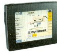
Portable terminals like this Case IH AFS Pro unit and other farm vehicles can be moved between different tractors.
