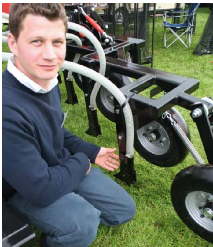
Jack Dale with the pivoting multi-tine coulters assembly on the latest All Till direct and minimum tillage seeder from John Dale Drills.
