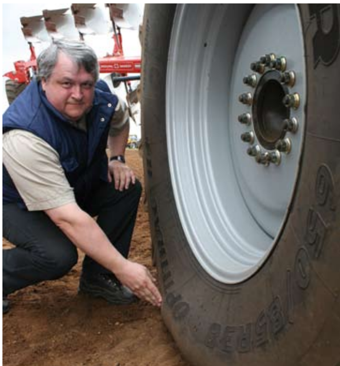
Mark Turner of Goodyear points out the tough but flexible sidewall that allows the Optitrac R+ to support heavy loads, but to operate at low inflation pressures.
