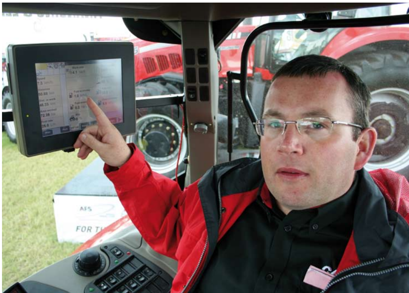
Information at your fingertips – Michael Gillon points out the numerous fuel consumption read-outs on the Case IH monitor available for Puma and other tractors.
