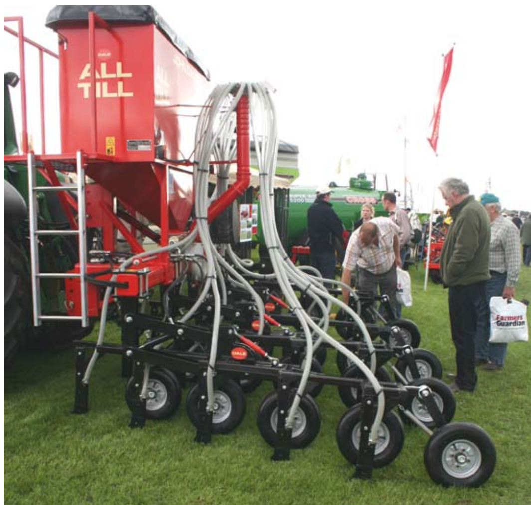
The All Till has a tall, slim hopper to keep the weight as far forward as possible. It holds about 1200kg of wheat and uses an Accord seed metering and distribution system.
