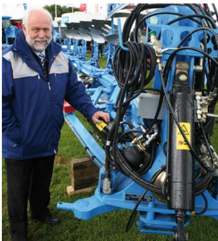
Lemken's Tom Hirst with the Tansanit "intelligent" plough. The key feature is the large hydraulic top link, which, under electronic control, transfers up to 2.5t to the tractor's rear axle to give it plenty of traction.
