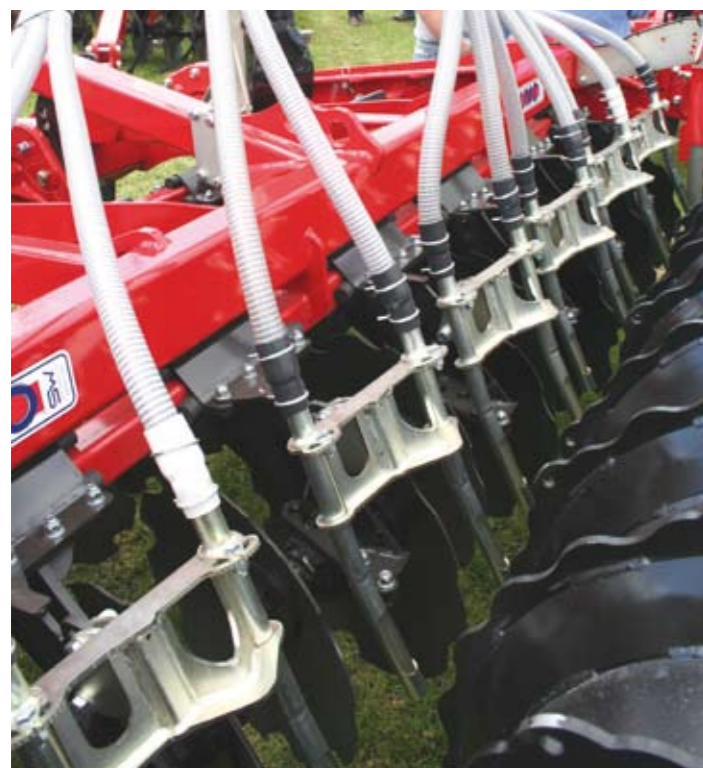
Seed is delivered by tubes into the shadow of each disc on the Sumo Trio D-spec cultivator-drill, where it is covered by soil thrown across by the adjacent disc. The Multipacker roller and finger harrow finish the process.
