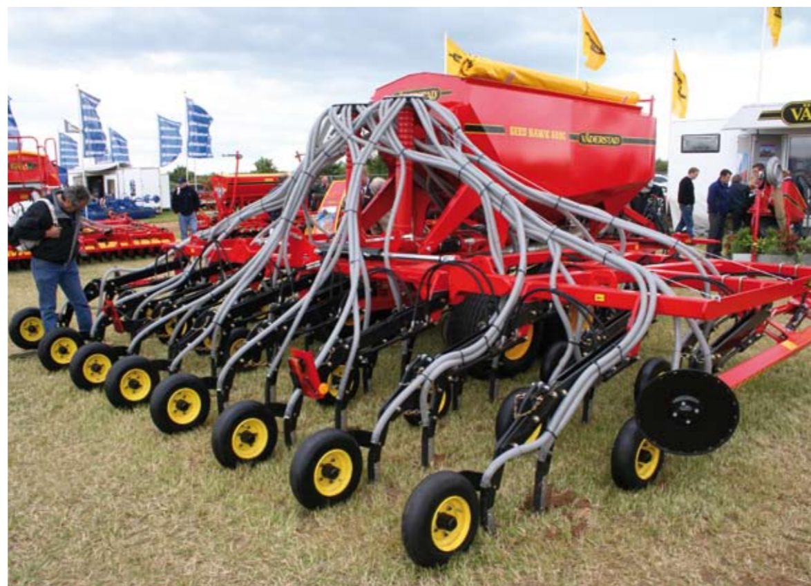
Seed is delivered by tubes into the shadow of each disc on the Sumo Trio D-spec cultivator-drill, where it is covered by soil thrown across by the adjacent disc. The Multipacker roller and finger harrow finish the process.
