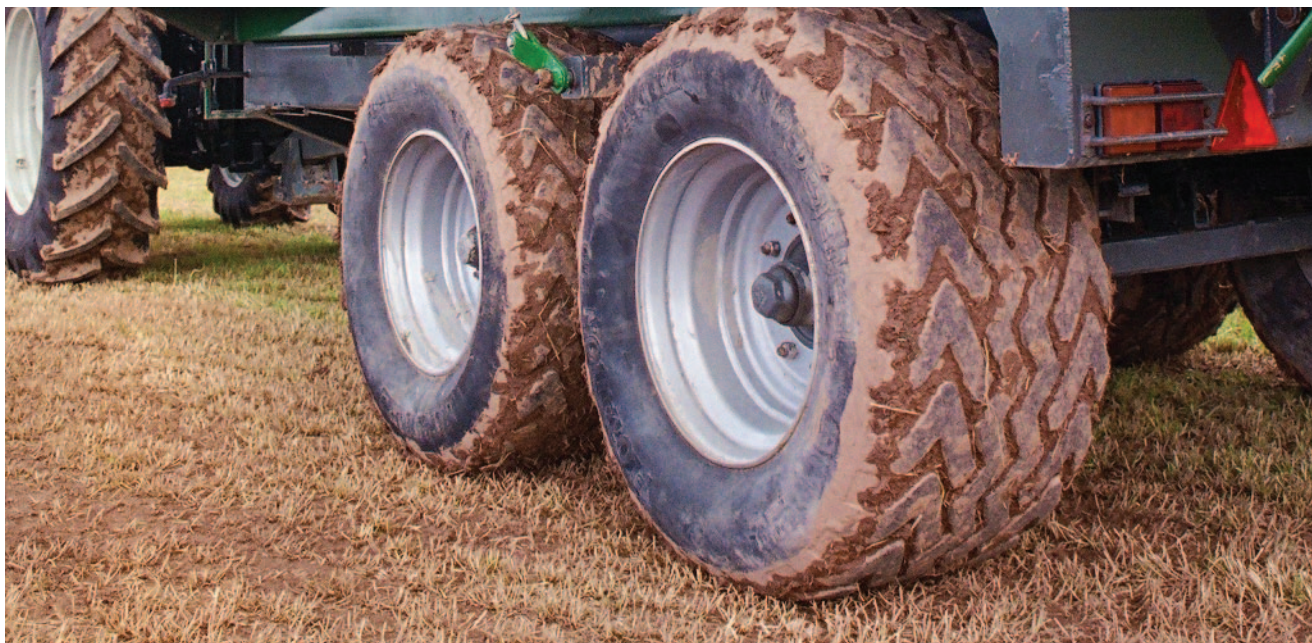
Big radial trailer tyres do not come cheap, but running costs can be lower than with tyres of inferior specification thanks to greater puncture resistance and making trailers easier to pull.
