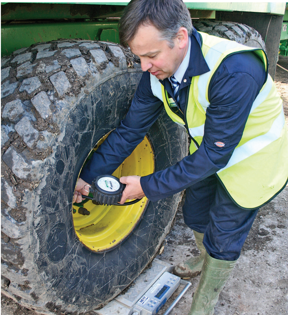
With trailer tyres, there is no real substitute for weighing to determine axle loads, so that the most appropriate inflation pressure for the tyres, load and operating conditions can be used.
