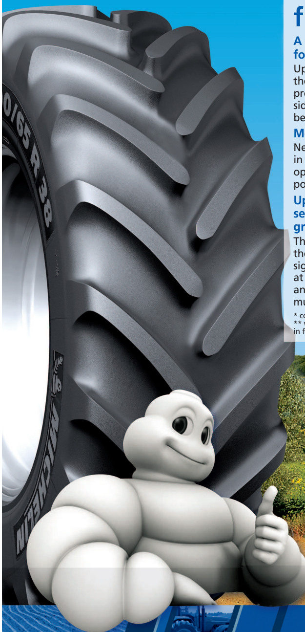
The advantage of using purpose-designed strong, but supple, radial tyres on silage trailers. In this case, 385/65R22.5 truck tyres in comparison with 500/60R22.5 Cargo X Bib on a pair of 14 tonne trailers.
