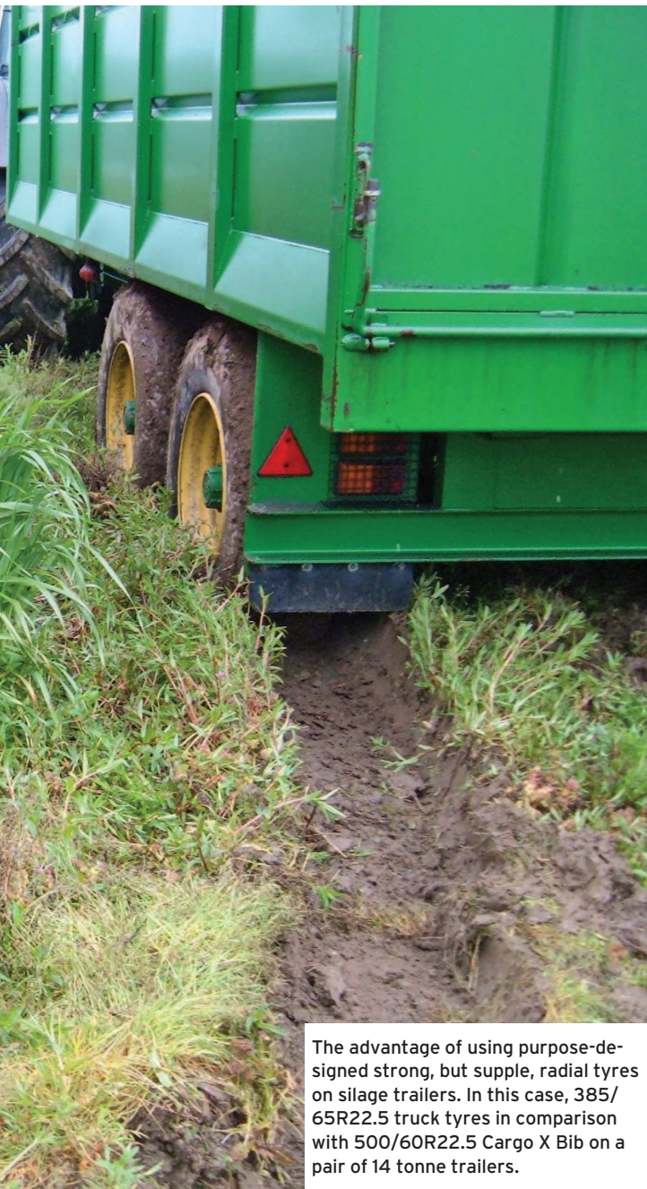
Big radial trailer tyres do not come cheap, but running costs can be lower than with tyres of inferior specification thanks to greater puncture resistance and making trailers easier to pull.
