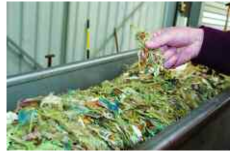
A specialist hammer mill takes in food deliveries, macerates the food and separates out the plastics with no manual intervention.
