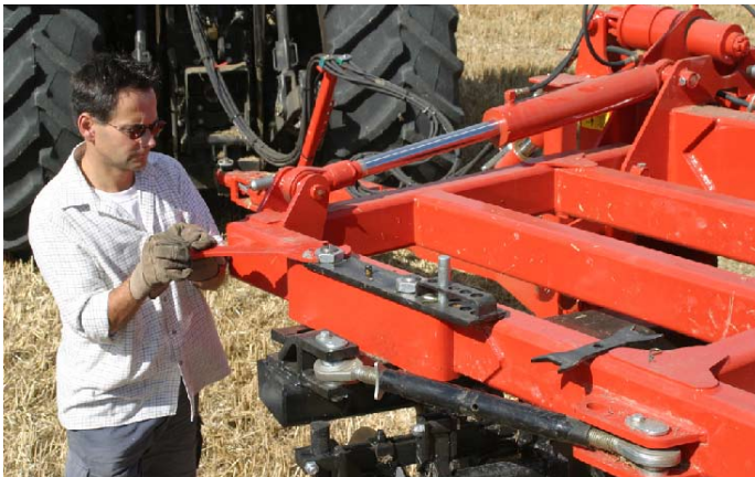
Only reason for adjusting front disc gang angle is to move more soil. Best advice is to leave this setting at the shallowest angle that still achieves the desired effect.
