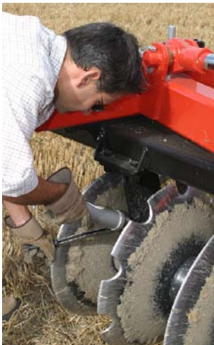
The daily maintenance on a 4.2m Discordon takes about 45-60mins - to grease all the disc bearings, wheels, chassis and pivot points. Auto-lube lists as a £2,100 option.
