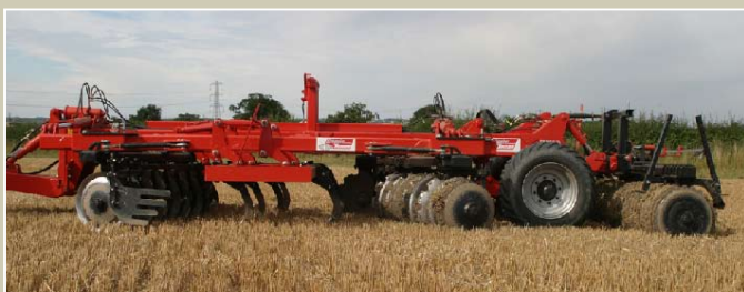
As with most machines of its type, the Discordon has a number of main working zones: Front discs move/loosen the soil, legs remove any pan, and rear discs mix, chop and level. The following press consolidates but it is not meant to be a surface-levelling tool.
