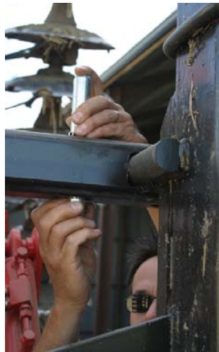
Packer locking pins should be inserted before heading out on to the road. We suspect that some operators simply will not bother.
