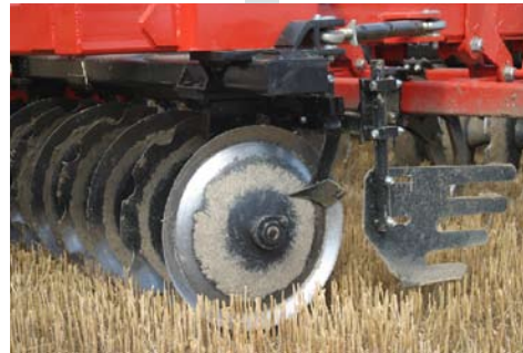
Only reason for adjusting front disc gang angle is to move more soil. Best advice is to leave this setting at the shallowest angle that still achieves the desired effect.
