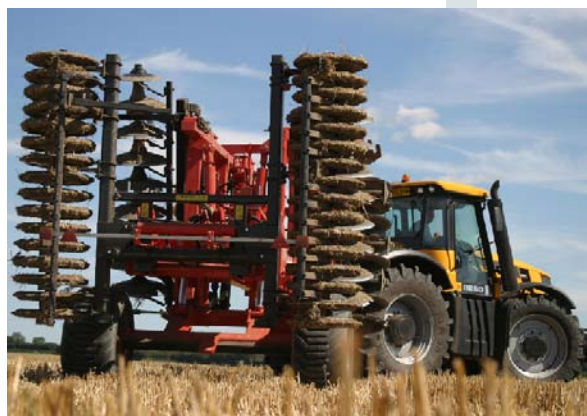
Discordon folds up to 3m for transport. One of the downsides of positioning the wheels right at the back of the machine is that manoeuvrability is compromised. Turning into tight field gateways can be a struggle.
