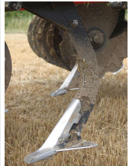
Discordon is no subsoiler. The lifting legs are designed to loosen the soil down to 150-250mm below discing depth – to remove any disc/plough pan.
