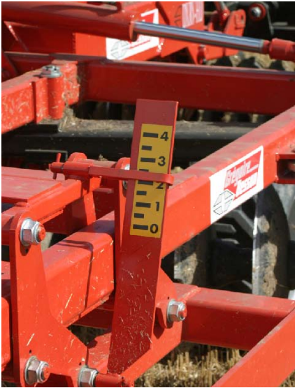
Depth of the legs can be controlled from the tractor cab on the move. Operator must check that the left and right wing sections are set at the same level.
