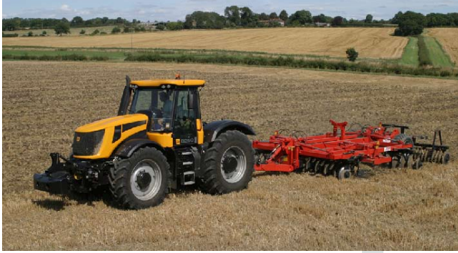
Tug for our test was a 185kW/248hp JCB Fastrac 8250. Shod with Pirelli TM800 710/70R38 rears and 540/65R38 fronts, the tractor hit our target 8.5-10.0km/hr travel speed under most conditions.
