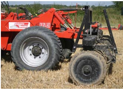
Rear linkage and rams provide the point of attachment for the packer. The 4.2m machine uses a two-part Emopak, whereas 4.7m+ units gain an extra section.
