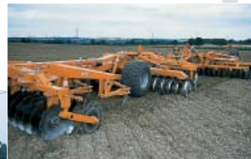
Our Simba Solo 300 configuration: 14 front discs, four soil loosening legs, intermediate row of 16 DD rings and ten rear discs. Trailed behind on our test train was a 4.6m wide DD double press.
