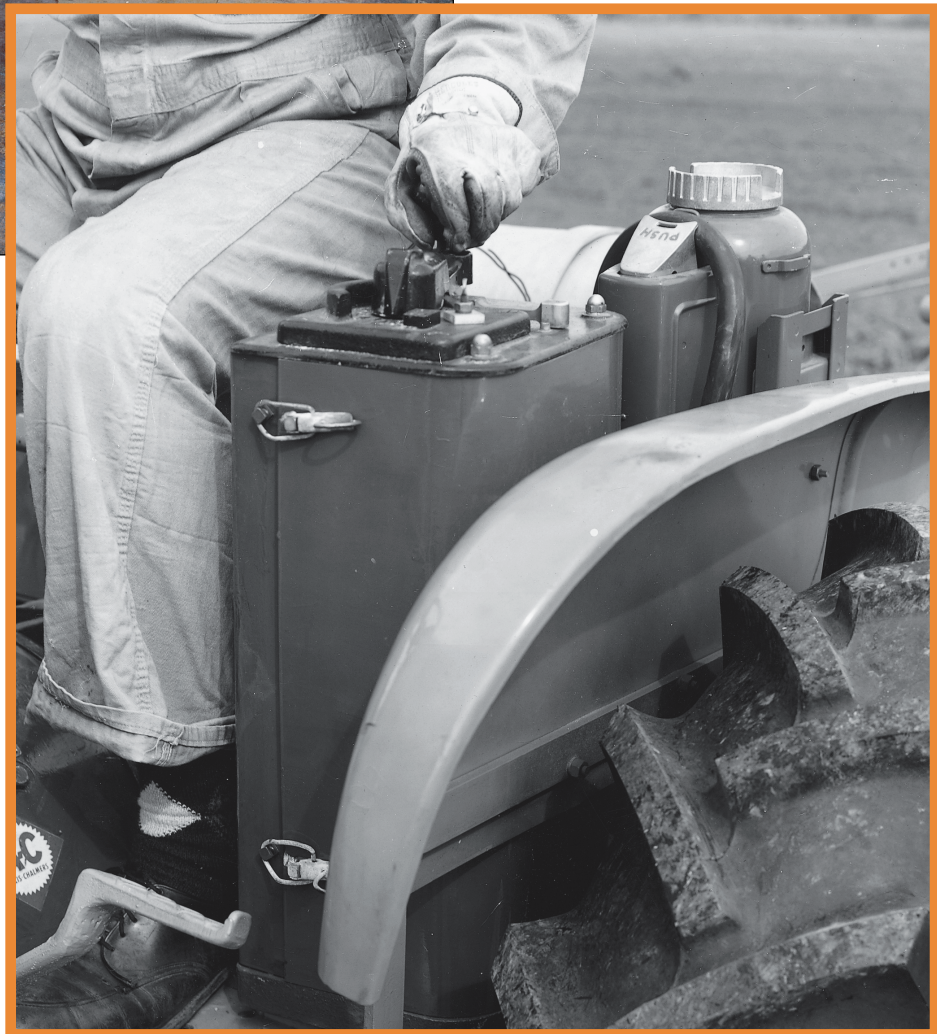
A small control panel by the driver's left hand side includes levers to adjust the power output and travel speed and for forward/reverse changes.
