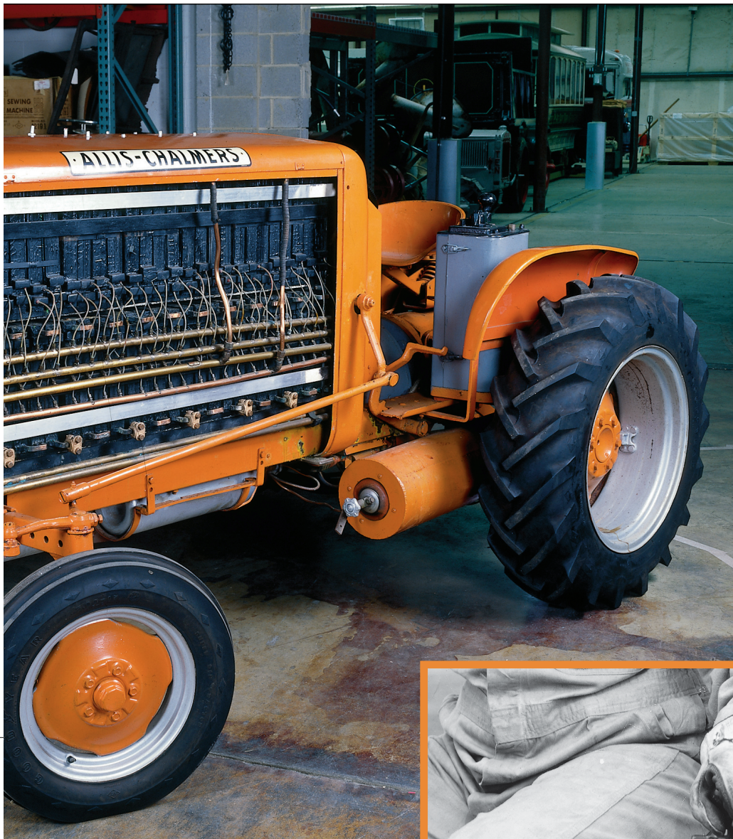
Above: The 1959 tractor photographed with the side panels removed to show the bulky fuel cells.
