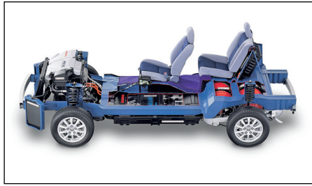
This cutaway view of Honda's FCX research vehicle shows how neatly a modern bank of fuel cells fits in a small family car.
