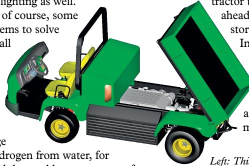
Left: This fuel cell powered Pro-Gator utility vehicle is part of a John Deere research programme to develop and evaluate electric vehicles and equipment.
