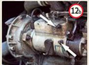
Start the air-bleed procedure by finding the lift pump (a) and injector pump bleed screws (arrows, b). On a 135 the lift pump is on the offside, the injector pump on the near.
