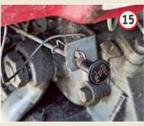
With the stop control in the 'run' position and the hand throttle opened up wide, spin the engine on the starter in ten second bursts until you see bubble-free fuel pulsing from the injector unions.
