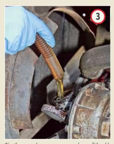
Give the sump plug a new copper washer, or if the old one is in good order, soften it by heating to cherry red and quenching in cold water. Replace the plug. Add fresh oil until just past the 'full' mark on the dipstick to allow for filter volume, then fire up the engine and check for leaks. Recheck the dipstick and top up.
