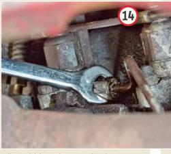
Follow each injector pipe up past the exhaust manifold; you're looking for the union nut where it joins the injector at cylinder head level. Using a short spanner, slacken each nut by a couple of flats.
