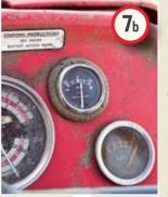
The dynamo or alternator drive belt needs to be in good order and tensioned properly; around 19mm (3/4in) deflection mid-way down a long belt run is good (7a). Slacken the unit's top pivot bolts a little, loosen the single anchor bolt underneath and swing it to adjust. Use a voltmeter or the tractor's ammeter to confirm a healthy charge (7b); a voltmeter connected between the battery terminals should show 13.5V-14.2V at medium rpm.
