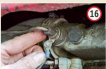
Cold-weather starting may be helped by a thermostart unit. This uses an electrical element and a dribble of diesel to make a little bonfire in the inlet manifold, warming the incoming air and combustion chambers. Check that it's working by holding the key in the 'heat' position for ten seconds but not cranking the engine; the base of the unit should get hot. Smoke from the air cleaner intake confirms thermostart operation.
