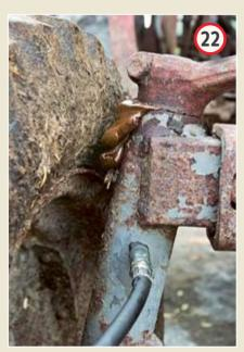
Grease every nipple you can find. If grease won't go in, swap the nipple for a new one. Key locations are front kingpins (picture) and the front axle's centre pivot. Pump away until water and old grease are driven out. Depending on the tractor, other grease points are on the steering joints, the steering column below the steering wheel, the brake pedal pivots, the front wheel hubs and the rear linkage lift rods.
