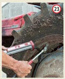
Finally, check the tyres. For a MF 135, the maximum pressure for 11.2x28 rear tyres is 14psi (4 ply) or 22psi (6 ply); for 6.00x19 front rubber it's 26psi.
