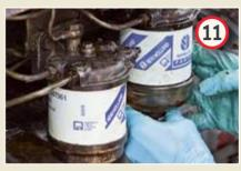
Fit the new filters, using the smaller square-section ring seal between filter and base. Tighten the holding bolt firmly, but don't go bananas or you'll do damage.
