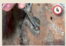
Transmission dipstick lives on the offside of the tractor, just ahead of the back axle. Oil should be up to the mark. If not, top up with a big-name brand Universal.
