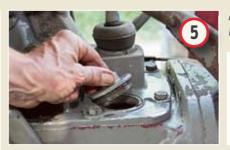
Add transmission oil through this big plug on top of the gearbox.
