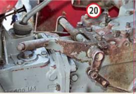
A working parking brake is not optional, it's essential. Adjust the brakes (see 19), then free off the handbrake linkage and lever button. On tractors with a pawl-type parking latch on the foot pedals, make sure the pawl is free to pivot and is effective at locking the pedals down. See that the parking brake holds on a slope, or you and your tractor could end up in the pit.
