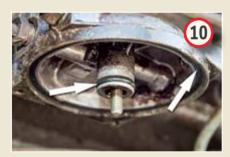
The filter head has two seals (arrows) which must be replaced, partly so the filter is not bypassed and partly to head off leaks. Replacements should come with the new filter; the bigger-diameter ring goes in the filter head. Grease the fresh seals and install, making sure neither is twisted. Grease holds the big seal in place.
