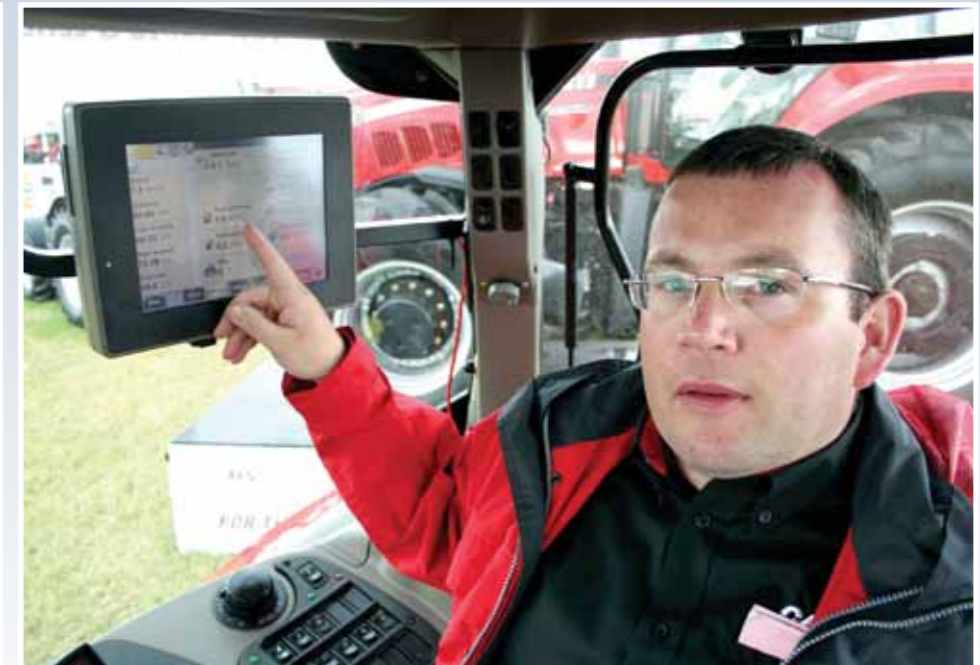
Above: Michael Gillon of Case IH points out the numerous fuel consumption read-outs that feature on the Case IH monitor available for Puma and other tractors.
